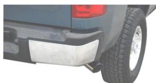
GIBSON EXHAUST systems are designed on a factory stock vehicle. Any aftermarket products installed could increase the sound levels of the exhaust. **Make sure there is a 1" clearance from ALL rubber brake lines, shock boots, lines, tires, etc. to prevent heat related damage or fire.**
