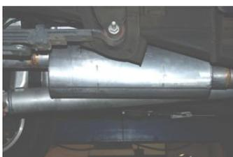
4. Install muffler #B onto headpipe #A 1 1/2"-2" with the louvers facing towards the converter. The outlet should be at the 11 o'clock position. Use a jack stand to support the muffler. Use clamp #E to secure the muffler to the headpipe. Do not tighten. Muffler inlet is looking into the louvers. Muffler outlet should be at the 3 o'clock position.
