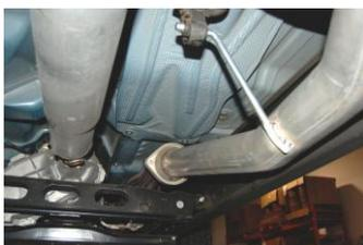
3. Install headpipe #A onto your existing stock front pipe using your factory nuts to secure. Do not tighten. Insert welded hangers into rubber grommets.
